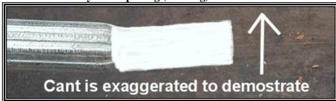
Insert **about twenty four (24) inches** of the tube end indicated by red paint (see tube orientation page) through the holding strap of the bender.
