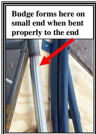
Lever bar show pulled back from small end of tube to better show the shoulder of small end
