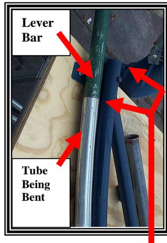
Every bending stroke should end about 5 inches from the end of the bender
