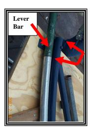
Ridge forms here, when finishing off the large end of tubing. It is created by the tip of small end of lever bar inserted into large end of tubing and bending pressure brings the two into contact with the bender body.
