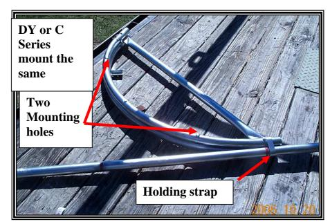
The following photos are of benders mounted in different ways. We recommend mounting your bender horizontally (flat) on a 4'x8' table or suitable flat surface.
