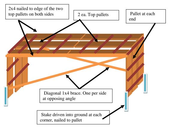
This pallet table does not require any plywood for the top. Just mount bender directly to the pallets in position shown for a plywood table top on page 3.
