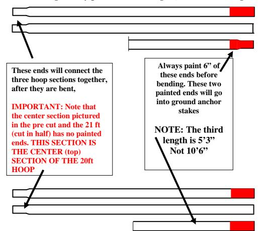
"B" Using factory 21 ft. lengths 1 3/8" 18 or 17 ga. cut in half. when cutting 21 ft lengths for this hoop there will be more than usual left over sections. use them for purling and connect them if necessary using the 1" x 8" lengths of emt described on pg 12.
