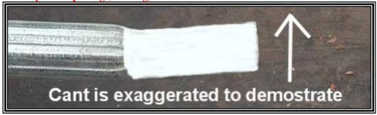
Insert about 4 inches inches of the tube end indicated by red paint (see tube orientation page) through the holding strap of the bender.
