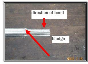
In this photo the junction of the lever bar and tubing should have been here, another 4 inches further back onto the bender. However at all times the completion of a bend on any tube, the junction of the lever and tube being bent must end on the bender body not past the bender. The action in above photo will be ok but it's getting to close the end of bender.
