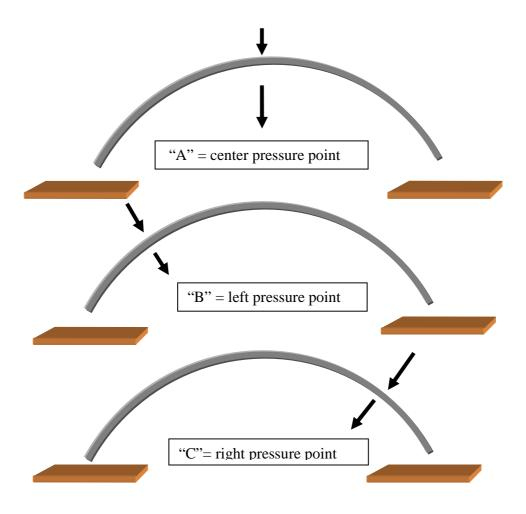
The three pressure points are the same regardless of section lengths sections. Applying pressure at these three points on each section and by allowing the ends to slide freely when pushing down, each section will uniformly be resized into wider hoops. After a few hoop sections this method will resize a section in about 20 seconds each. AGAIN, NEVER attempt to resize using any other method or press down in more places other than the three points shown above.
