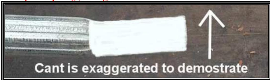
Insert **about 4 inches** of the tube end indicated by red paint (see tube orientation page) through the holding strap of the bender.
