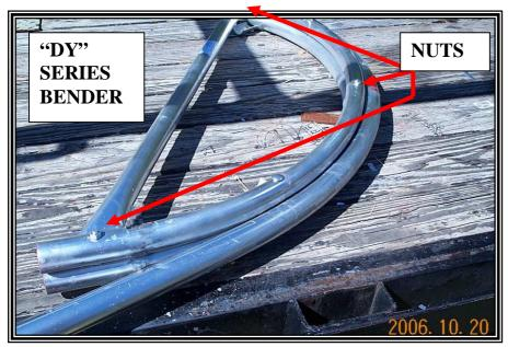
I will show you several different methods of mounting your bender in the following pages. The mounting table can be anything that is at the proper work height and will not move as you bend the tubing. The mounting table doesn't need to be elaborate. In fact the first example is a simple and effective table constructed with four wooded pallets shown below in the drawing, two 8 ft. 2x4s and a few 1x4 boards.
