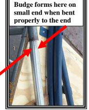
Lever bar show pulled back from small end of tube to better show the shoulder of small end
