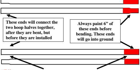
"B" Using factory 21 ft. lengths 1 3/8" 18 or 17 ga. cut in half.
