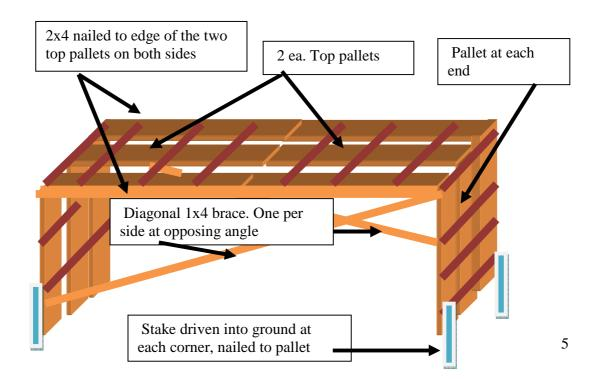
This pallet table does not require any plywood for the top. Just mount bender directly to the pallets in position shown for a plywood table top on page 3.
