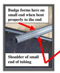
Budge shown above, tubing shown is armadillo Brand tubing and is fluted tubing not smooth as is most.
