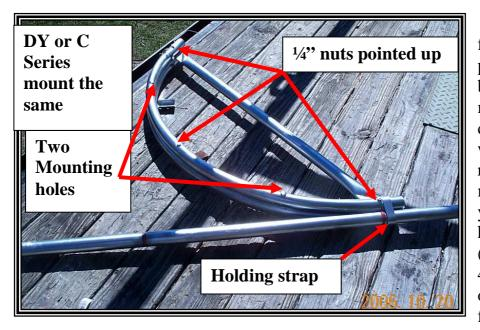
The following photos are of benders mounted in different ways. We recommend mounting your bender horizontally (flat) on a 4'x8' table or suitable flat surface. In the photos it is simply lag bolted to a flat bed truck. The bender body is held together with three  $\frac{1}{4}$ " carriage bolts, Be sure the side of the bender that faces up, is the side with the three  $\frac{1}{4}$ " nuts.
