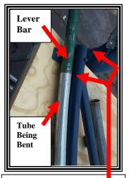
Every bending stroke should end about 5 inches from the end of the bender
