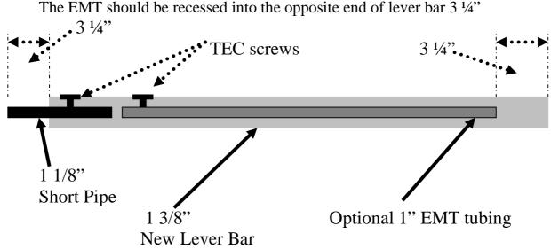
The EMT should be recessed into the opposite end of lever bar  $3\frac{1}{4}$ "
