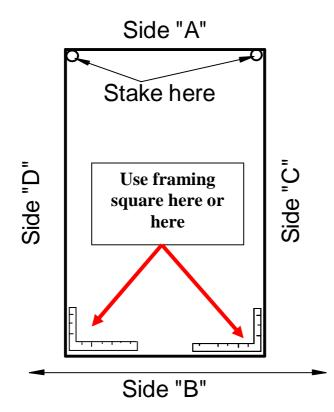
Side "A" is anchored with the two permanent 1 5/8" Tubing stakes, and then temporally fastened to the stakes.
