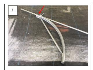
Position tubing with end mark just showing through the clamp
