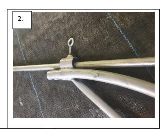
Mark each 10' length of tubing at 5' (center) Also using the table below for your model bender-mark each tube at the prescribed distance from each end.
