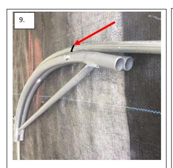
In this photo you can see the 5' mark. And because I want to bend the tubing a few more inches past this mark I release the pressure, slide tubing through the clamp another 8" to 10" the make a short quick third stroke as seen in photo #10.
