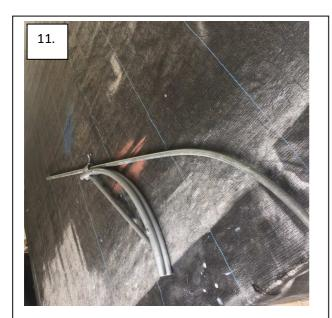
Flip the tubing end for end (change ends) and slide the other end through the clamp, stopping at the prescribed distance as for your model on the other end of tubing.
