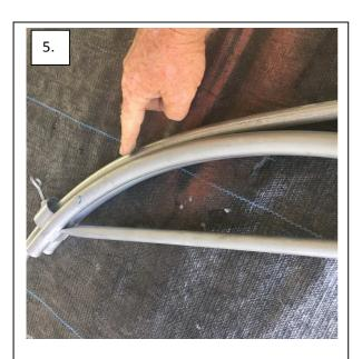
Release pressure & slide the bent portion through the clamp. Make sure to leave 7" or 8" of the bent portion on operators side of the clamp before beginning the second bending stroke.
