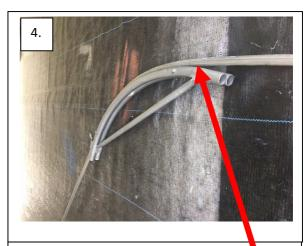
Pull tube around the bender stopping 4" before reaching end of the bender.
